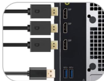
2. Connect KVM's DP output ports to 3 DP displays with 3 DP cables.
