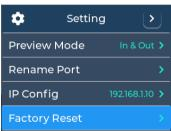
**Tips:** 1. When you want to return to the previous menu level, you can press the ":≡" button to return, or you can rotate the dial to the return button at the top right of the LCD and press to return.
