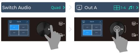
**Tips**: Before using this function, make sure that at least one output showing Quad-view is currently available.
