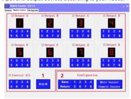
**Tips:** 1. The digital number 1-8 means input 1-8. And **9** means 1~4 Quad-View, **A** means 5~8 Quad-View
