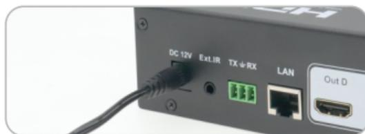
5. By now, the connection has been completed. Turn on the power supply and the HDMI Matrix will begin to work.
