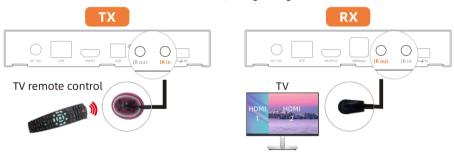
Signal Flow: TX-side remote control  $\rightarrow$  commands  $\rightarrow$  RX-side display.
