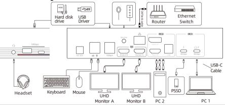
**Tips:** For optimal performance, use the included Thunderbolt 4 cable to connect the PC and the original Thunderbolt 4 cable to connect the PSSD.
