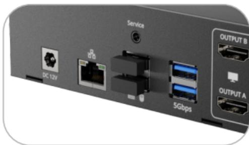
6. Connect USB 3.0 devices to KVM's standard USB 3.2 ports.
