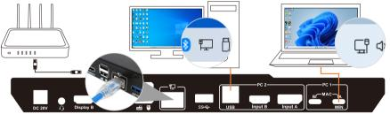
**Tips:** It is recommended to connect the USB cable to a USB 3.0 or higher port on the PC to achieve a Gigabit bandwidth network connection.
