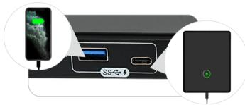
Use the USB ports on the front panel of the KVM (including an USB-A and an USB-C ports) can support data transmission while charging. The USB port support BC 1.2 protocol, and are able to match voltage and current automatically based on the specifications of charging devices. It makes your charging safe and avoid damage.
