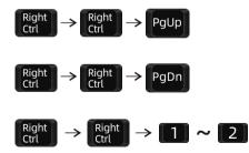
Switch PCs on different monitors separately(i.e. display mode 2): Monitor 1: [Right-Ctrl]  $\rightarrow$  [Right-Ctrl]  $\rightarrow$  [ $\leftarrow$ ]  $\rightarrow$  [1]~[2]
