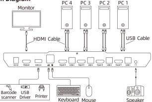
**Tips:** The PC 1 and PC 2 here refer to common HDMI input devices. That's to say, TV Box, Amazon Fire TV Stick, Sky Q Box and other gaming devices can also be connected to this KVM.
