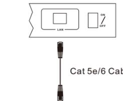
Connect to local area network router or directly to PC
