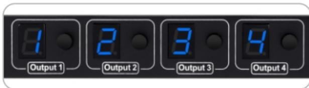
The digital display shows the input port number selected by the current output port, and the button beside every digital display is the input selection button.
