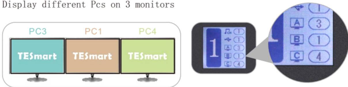
In this mode, each input and output port on the KVM is marked with a letter, and the screen corresponding to the output port is output by the port with the corresponding letter of the PC selected. As shown in the figure above, the screen output by the monitor connected to Output A is from Input A of PC 3, the screen on Output B is from Input B of PC 1, and the screen on Output C is from Input C of PC 4.
