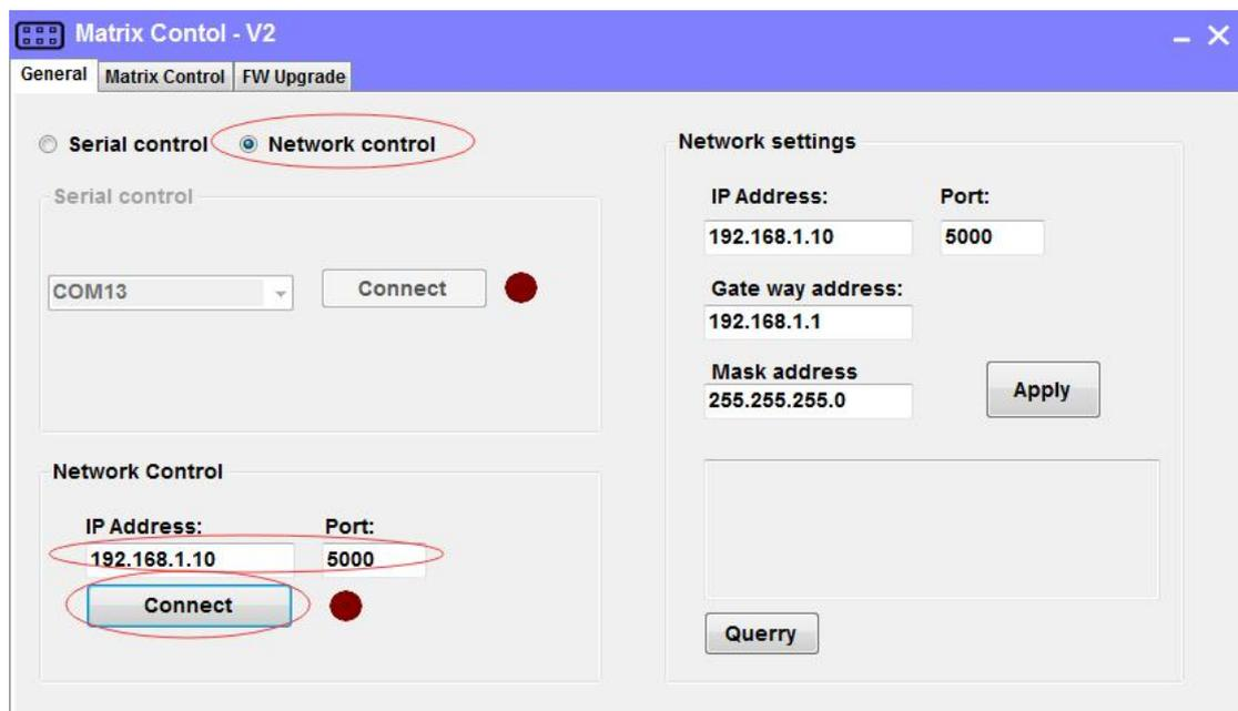
4. In "Network settings" area, modify the IP address settings as you want, but make sure IP Address and the Gate way address should be in same subnet. Then press "Apply" button to final submit the modification request. If succeed, the modified IP address will be displayed automatically on the information area. Power off and on again, the matrix will use new IP address.
