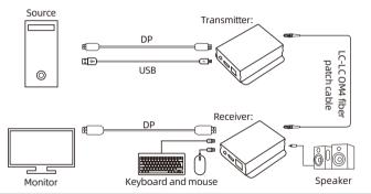
Tips: 1. Ensure LC-terminated multimode fiber meets IEC 60793-2-10 specifications for OM4 performance.
