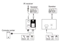
**Step 4:** Directly connect the DCCI port of first KVM switch according to above steps, in order to realize simultaneous display of 4 monitors
