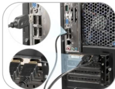
3. Connect external mouse and keyboard to KVM's keyboard and mouse input port.
