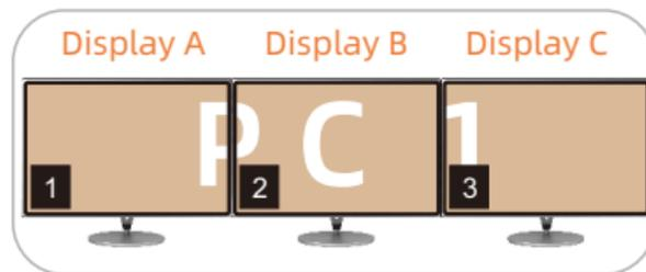
**Tips:** 1. If a device that doesn't support MST is connected, the display will only show on output A or show three duplicated screens. The specific situation depends on the device.
