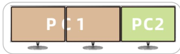
In this mode, you can show one PC on any two monitors connected to the KVM and the other PC on the remaining monitor. Use the front panel, hotkeys, or IR control to switch between PCs and monitors.
