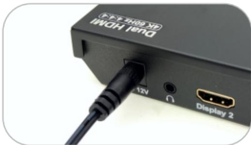
7. By now, the connection has been completed. Turn on the power supply and the KVM Switch will begin to work.
