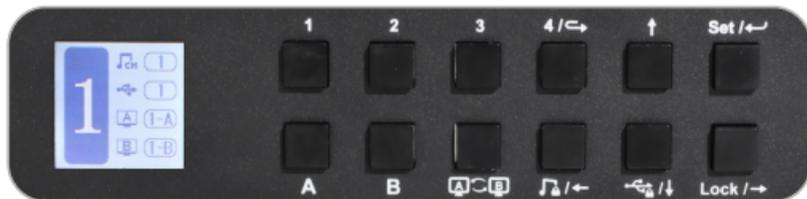
When you use the front panel button or IR remote to control the KVM, the LCD display will inquiry your target action, then execute the command according to your operation. The LCD interface in the figure above is the main interface.
