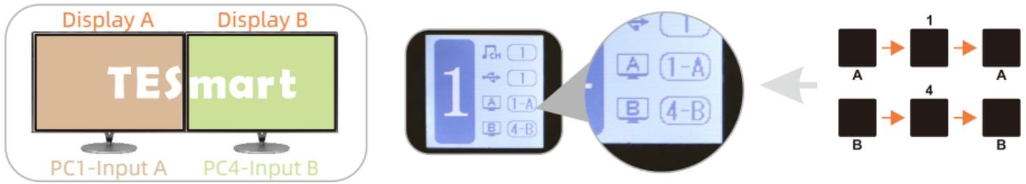
The selected Input A/B are correspondingly displayed on Display A/B.
