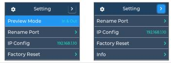
**Tips:** 1. When you want to return to the previous menu level, you can press the ":≡" button to return, or you can rotate the dial to the return button at the top right of the LCD and press to return.
