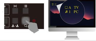
**Tips**: After pressing the button, the display OSD will not be displayed all at once, but will appear on each monitor in turn. When switching, only the switched monitor will show OSD.
